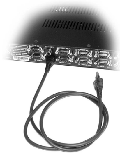
Optical cable (to connect equipment with optical output connection)
